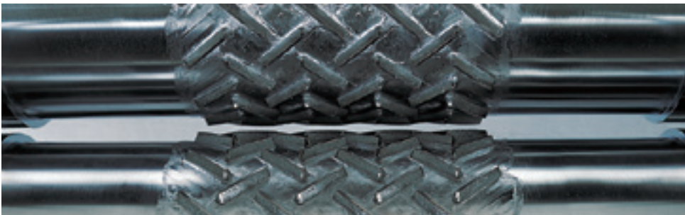
Embossing/embossing (Tip to tip unevenness)
